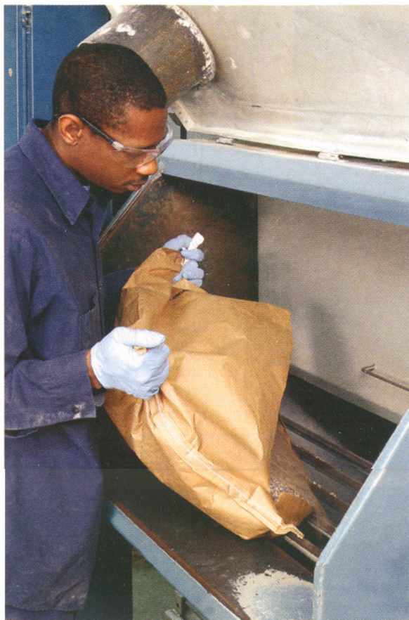
An access panel on the side of the rotary batch mixer provides easy access for personnel to perform cleaning and maintenance.
