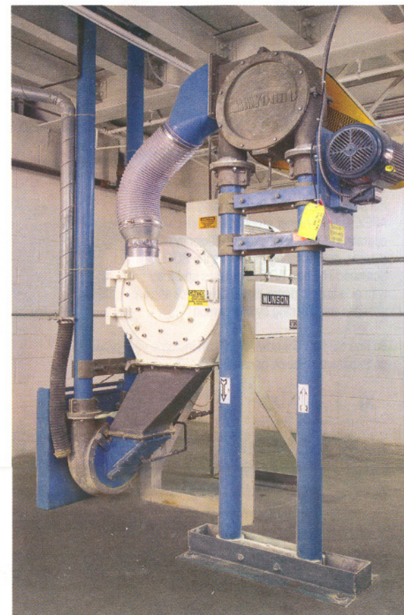
Fine powders are processed in this attrition mill (center left) and pneumatically conveyed to the packaging area via the blue tube at the left.
